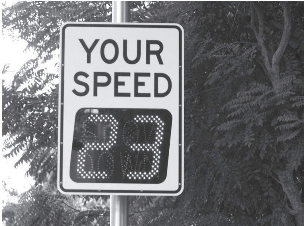
Figure 2: Picture of Speed Feedback Sign
